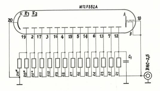
Fig. 1 Circuit diagram for M12FS52A
