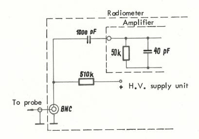
Fig. 2 Input circuit
